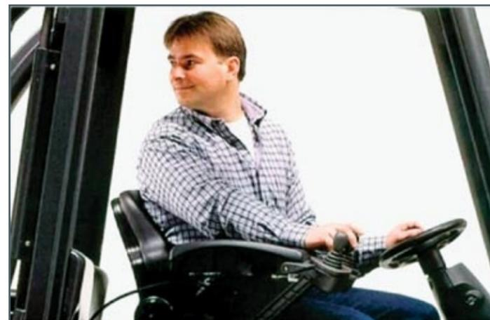
All controls located for easy and intuitive use. The operator's seat can be swivelled 17° to the right for every reversing manoeuvre.
